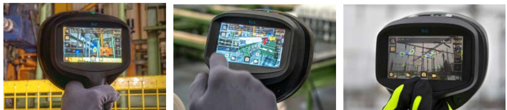
Ultrasound cameras showing, from left to right: compressed air leak, mechanical fault, and partial discharge.
